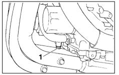
1. Coolant drain bolt
